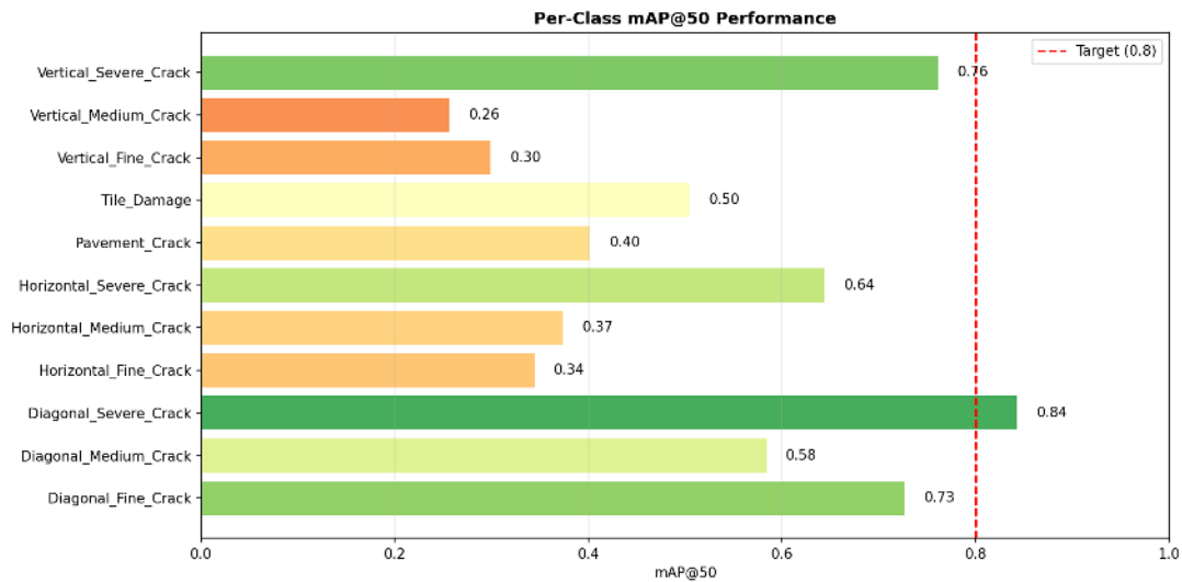
Figure 4: Per-class mAP@50 performance showing variation across the 11 crack categories. The red dashed line indicates the 0.8 industrial threshold.
