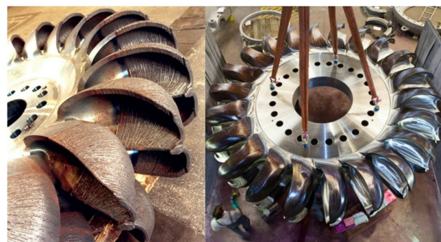
Fig. 25 Pelton turbine runner fabricated using Wire Arc AM [133, 134]
